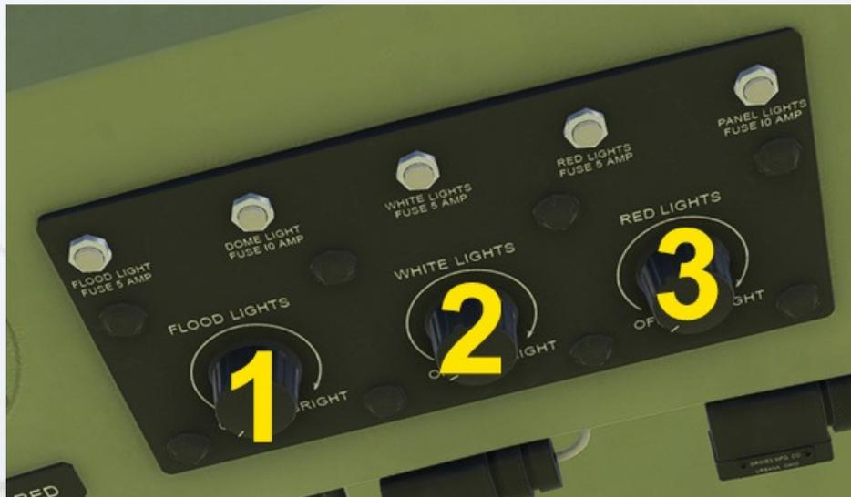
**1. Flight Engineers' Dome Light** - Controls the light intensity of the Flight Engineers' left side dome light. Dome lights are set to white only.
