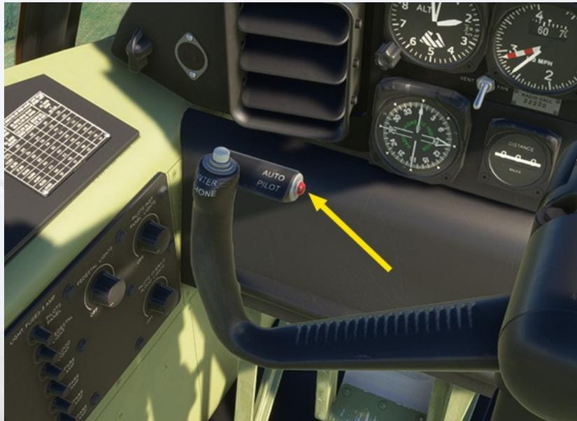
The position of the switch gives an easy visual check of the on/off status of the autopilot : in = ON, out = OFF.
